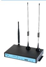
GSF 4363 ROUTER is a cellular terminal device that provides data transfer function by WCDMA/HSDPA/HSUPA/HSPA+ network. It can conveniently and transparently connect your existing Serial and Ethernet devices to a cellular network
